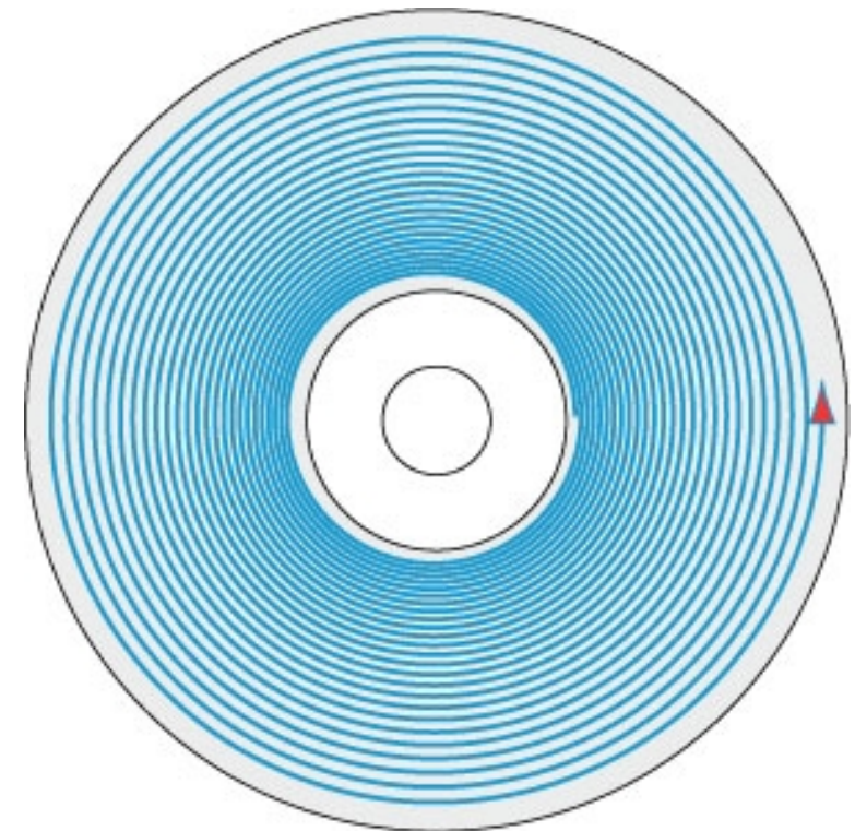
Spiral Data Track on Optical Discs (CD, DVD and High Definition Discs)
